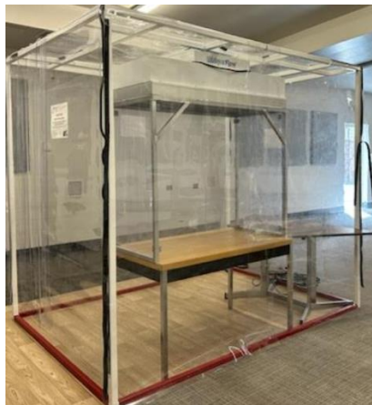
Figure 11: Current Cleanroom Design
