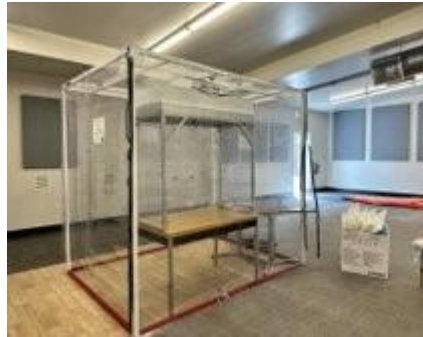
Figure 1: Current Cleanroom Design
